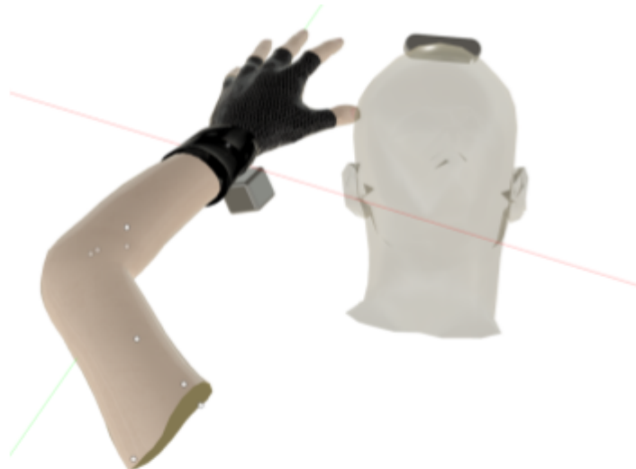
Figure 4: Wrist mount with Intel RealSense, Chi Et Al's Stereo Mirror, glove, and head mounted Intel D435 positioning
